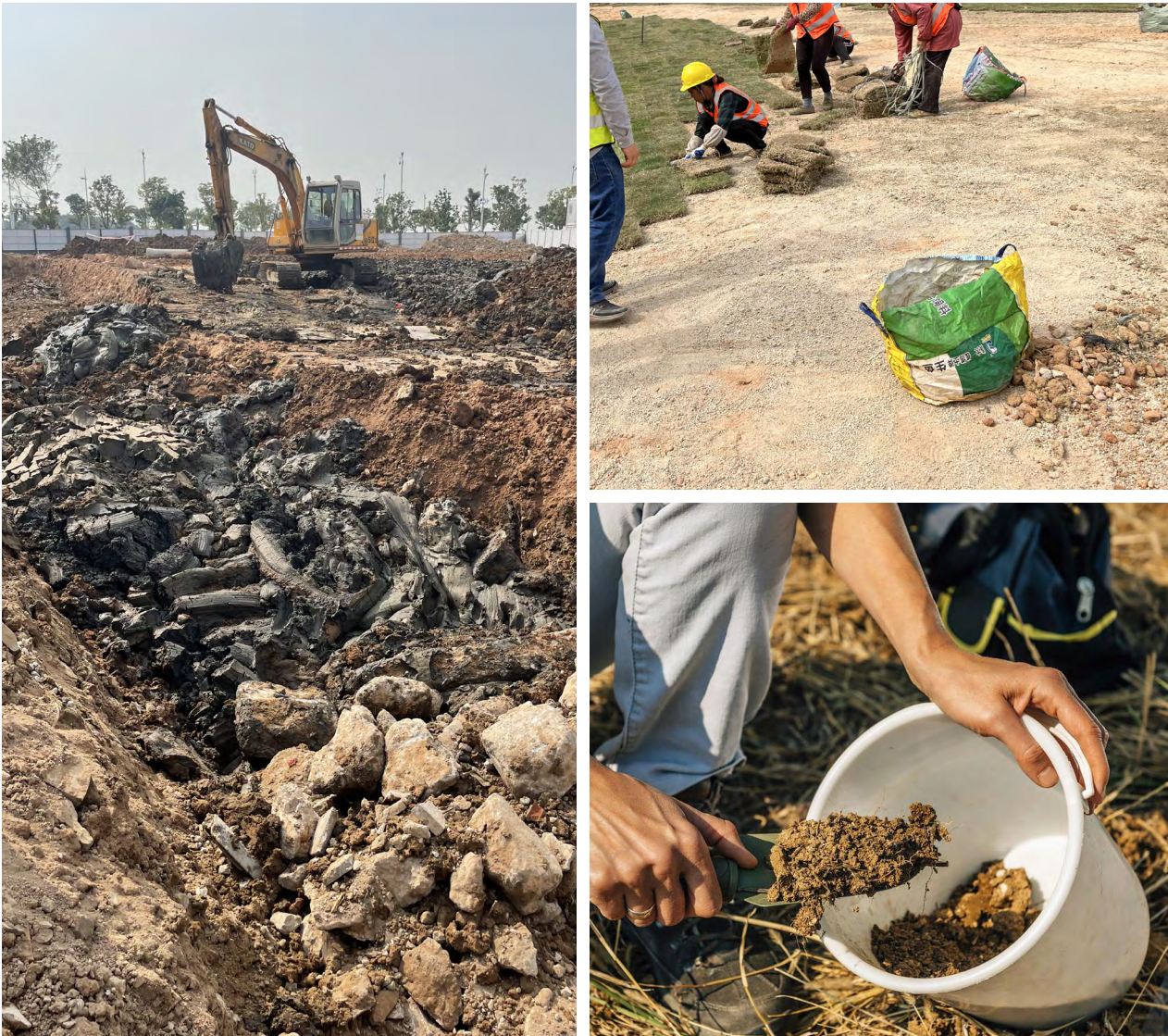
Soil at the site was collected and sampled to test EC value, pH value, salt content and permeability. The results will guide us to better modify the soil to make it more suitable for plant growth.
