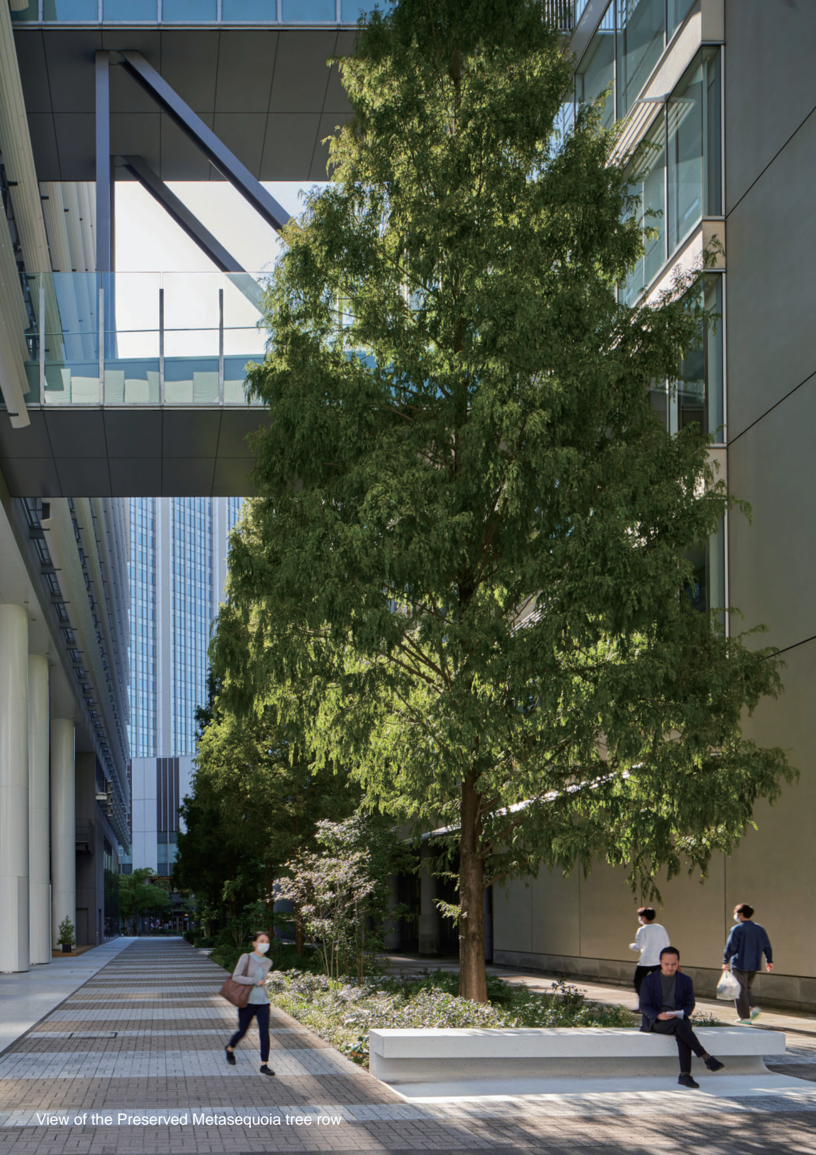
Widening of plantings at the foot of existing trees to prevent roots from breaking paving blocks
