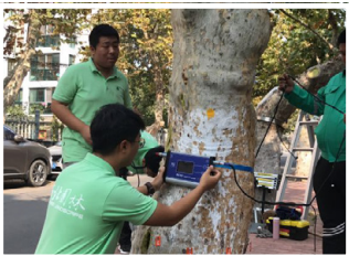
Monitoring of tree damage (Acoustic wave detector for tree cross section)
