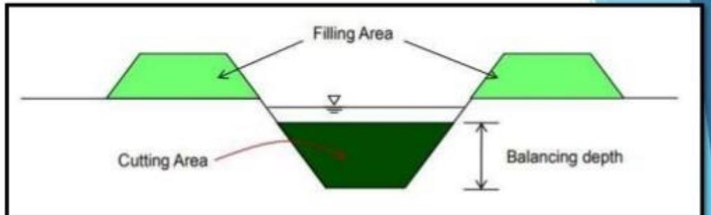
If for a channel section the depth of cutting is such that the quantity of excavation or cutting is equal to the earth filling required for making the banks, then depth of cutting is known as balancing depth or most economical depth of cutting.
