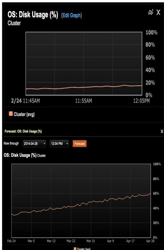
Figure 5 – An example of using OpsCenter to monitor and forecast used disk space
