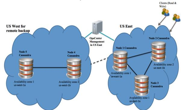
Figure 4 – Setting up a multiple DC configuration for backup or disaster recovery
