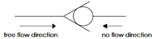
**Figure 1.1** Graphical symbol of a check valve.
