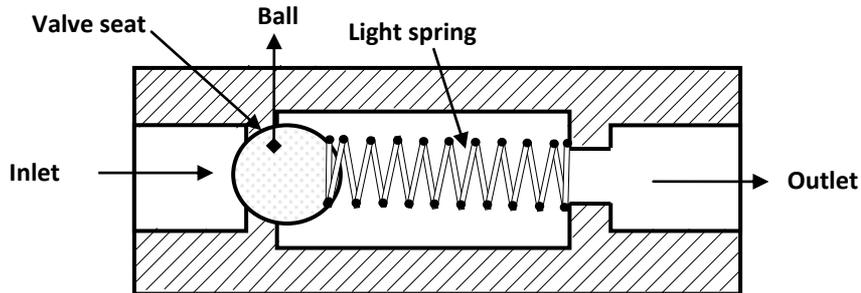
**Figure 1.2** Ball-type check valve.
