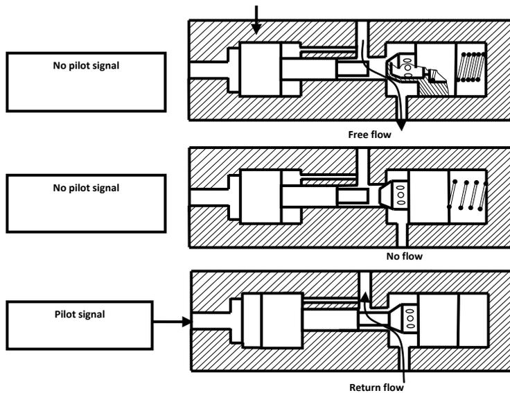
Figure 1.4 Pilot-operated check valve
