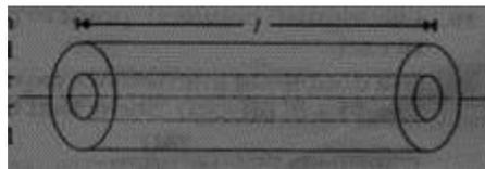
section  $A$  and number of turns/length  $n_1$ . The corresponding values for the inner solenoid are  $A_2$  and  $n_2$ . Write the expression for the inner solenoid are  $A_2$  and  $n_2$ . Write the expression for self inductance  $L_1, L_2$  of the two coils and their mutual inductance  $M$ . Hence show that  $M < \sqrt{L_1 L_2}$ .
