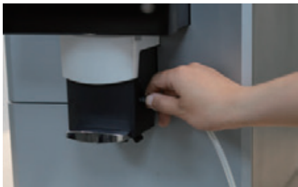
1. Connect milk pipe to machine
