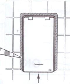
Don't apply sealant at the bottom side.
