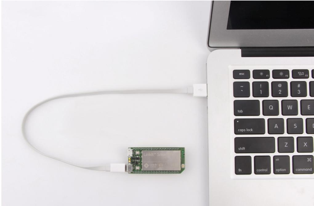
**Figure 1 Providing power to the LinkIt Smart 7688 board**
