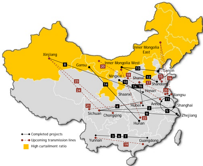
Fig 29: China high voltage transmission line construction plan
