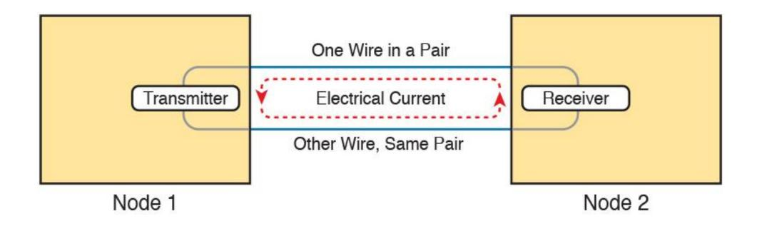
Building Physical Ethernet Networks with UTP Breaking Down a UTP Ethernet Link
