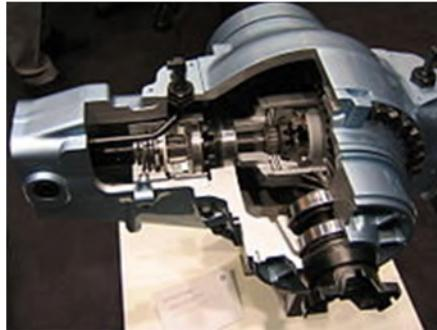
Figure 2. The drive shaft enters from the front and the driven axles run left and right
