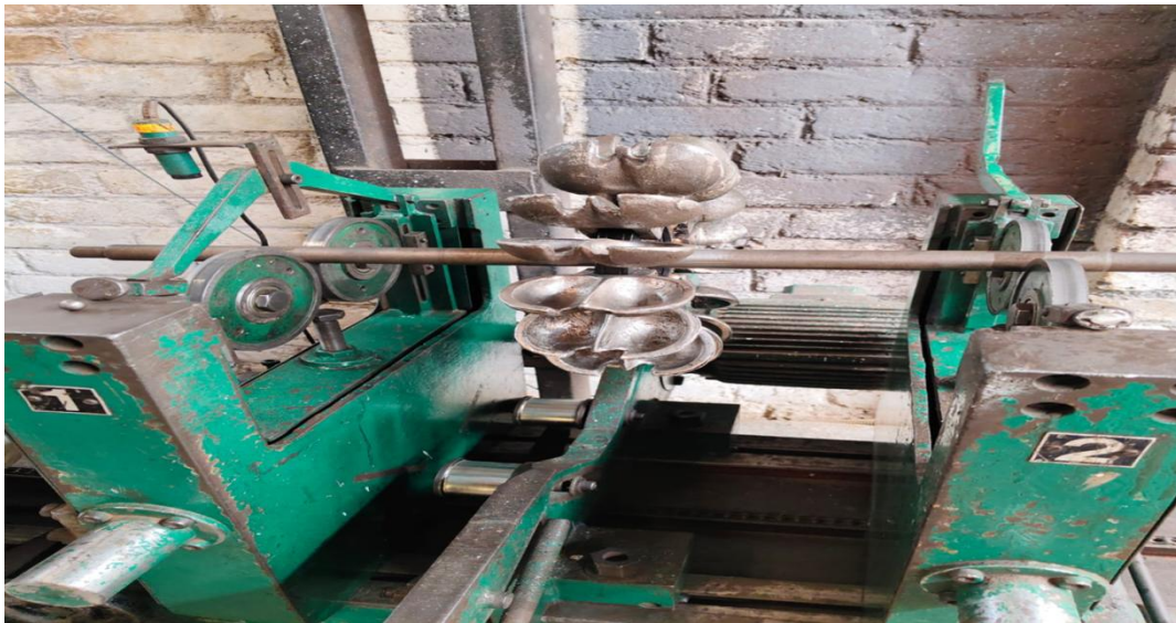
Figure 6.10 Dynamic balancing setup of Pelton turbine runner
