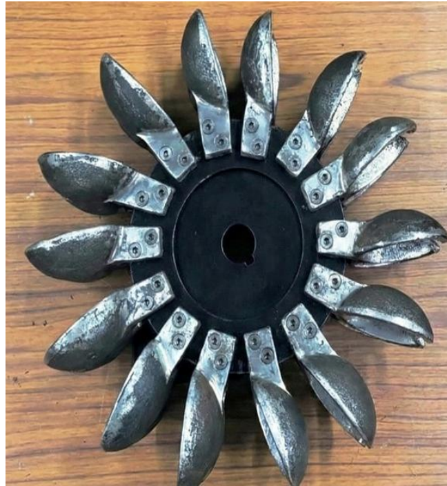
Figure 6.9 Bucket mounting arrangement
