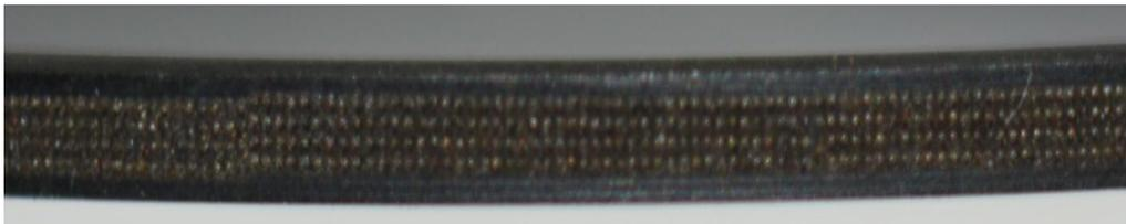
LST in the center portion of piston ring (Partial LST)
