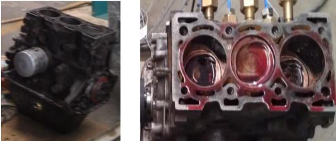
Photo-3 Maruti 800 C.C. 3-cylinder inline petrol Engine (Front view & Top view)
