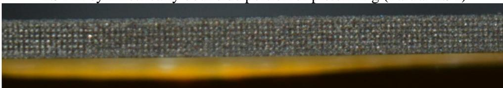
LST on the full-width portion of piston ring (full LST)
