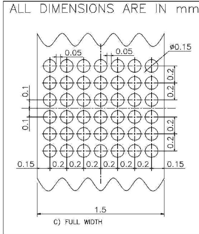
Figure 2. Drawing of LST Pattern on piston ring
