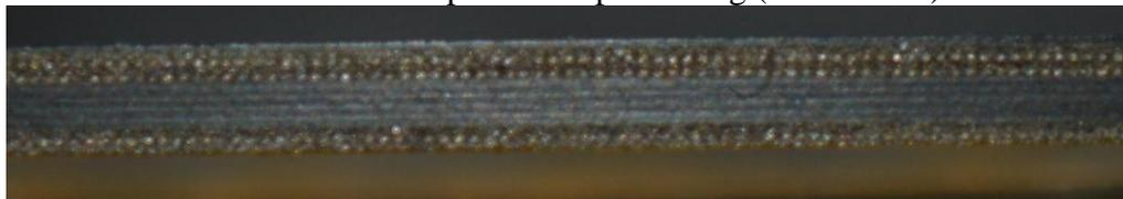
LST in symmetrically both side portion of piston ring (Partial LST)
