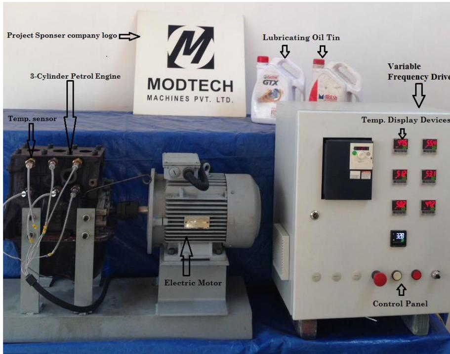
Photo-1. A photographic view of Actual Multi-Cylinder Engine Test Rig
