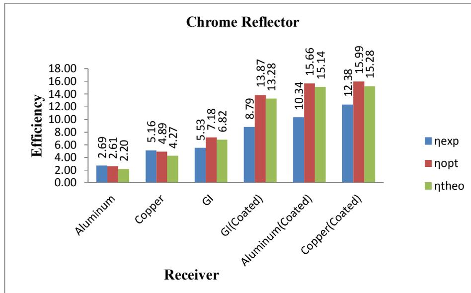
Figure 6 Graph of Average efficiency of Collector with Chrome Reflector
