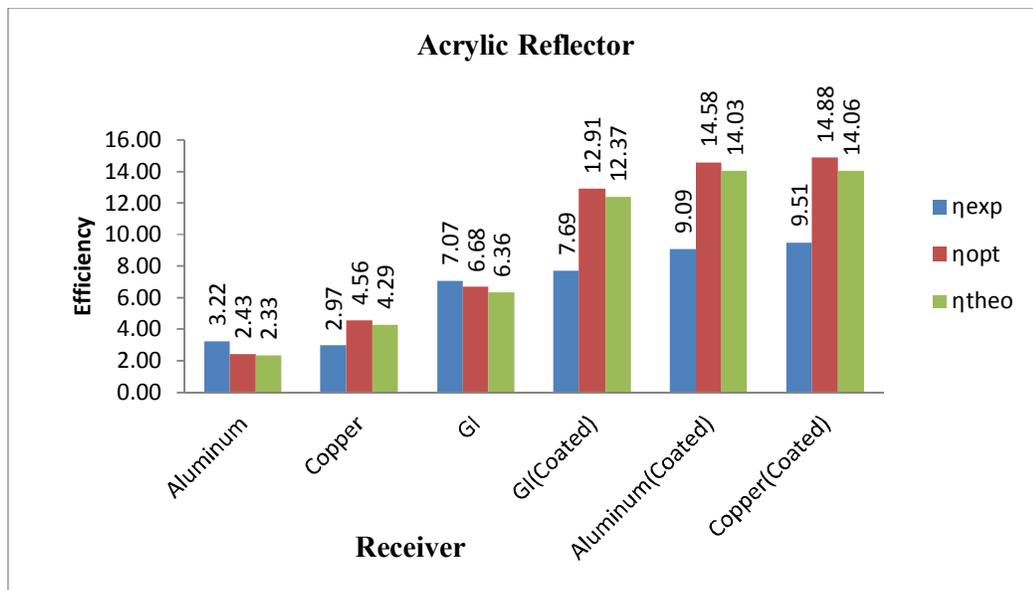
Figure 8 Graph of Average efficiency of Collector with Acrylic Reflector
