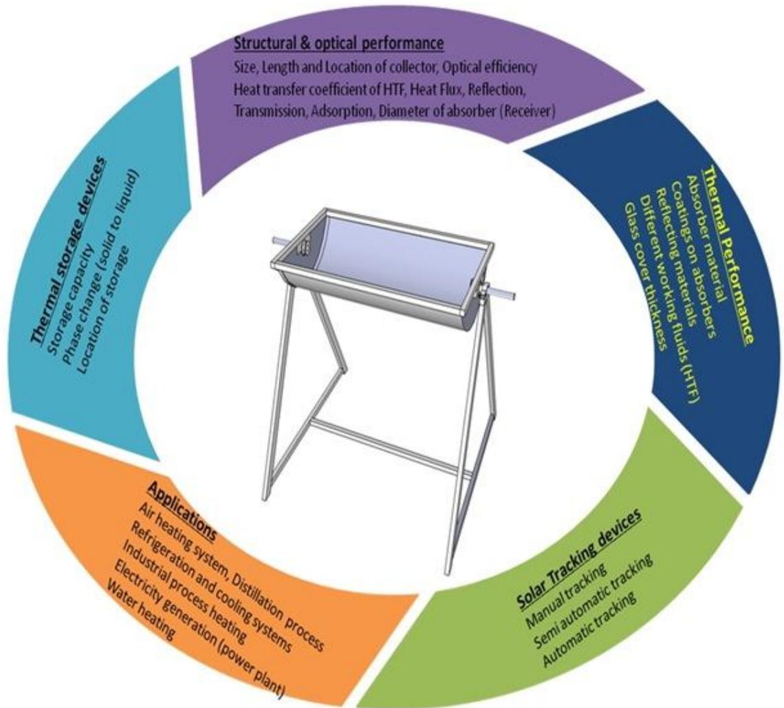
Figure 1 Key parameters of PTC
