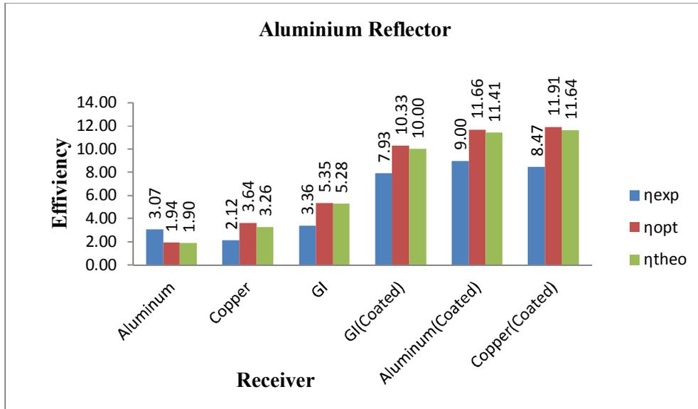
Figure 7 Graph of Average efficiency of Collector with Aluminium Reflector
