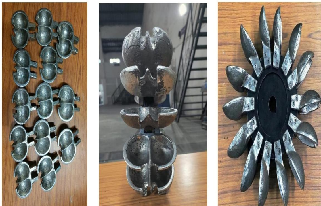
Figure 5 Fabricated Stainless Steel 314 enhanced Pelton bucket — individual buckets (left), buckets fitted on runner disc (centre), and completed 14-bucket runner assembly (right)
