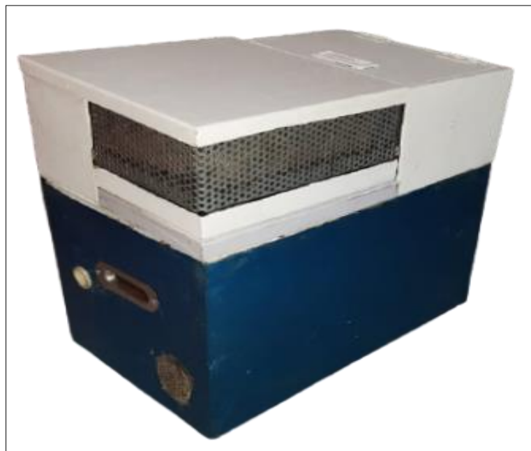
Fig. 6. Complete prototype of evaporative cooling based BTMS
