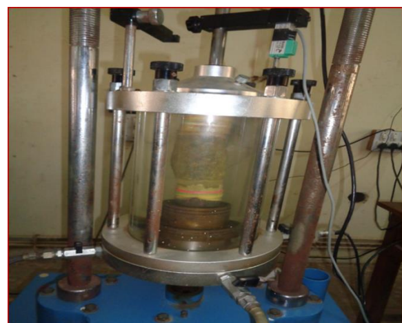
Sample-30% clay+ 70% gravel (during testing)
