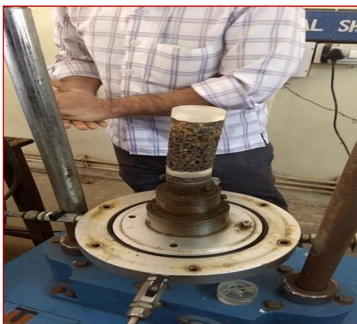
Fig. 2 Sample-30% clay+ 70% gravel (before testing)
