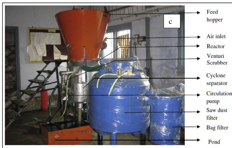
FIGURE 5.1.1.1: First, drawings of the downdraft gasifier (in cm) (a), second, gasifier in downstream system (b), and the picture of the installed unit gas cooling and cleaning systems (c).
