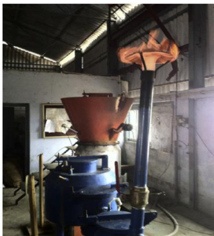
FIGURE 5.1.1.2: Burning flame of producer gas in gasifier.
