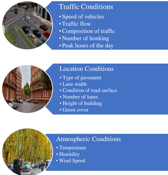
Figure 2.1 Factors affecting traffic induced noise level
