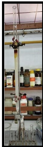
FIGURE 3.2, Column chromatography of P. corylifolia seed extract
