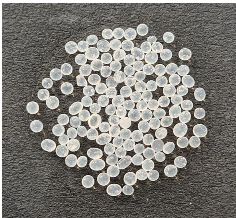
FIGURE 3. 6 Actual image of Silica gel solid desiccant used for experimentation.
