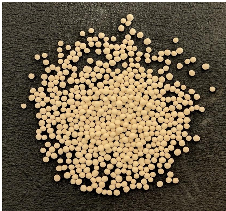
FIGURE 3. 7 Actual image of Molecular Sieve 3A solid desiccant used for experimentation.
