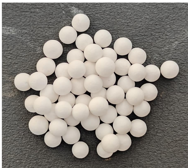
FIGURE 3. 9 Actual image of Molecular Sieve 13x of solid desiccant used for experimentation.
