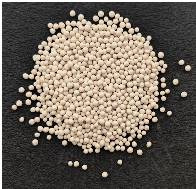
FIGURE 3. 9 Actual image of Molecular Sieve 13x of solid desiccant used for experimentation.
