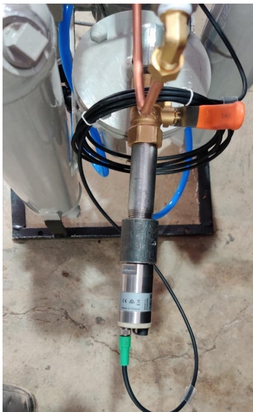
FIGURE 3. 19 Dew point meter for testing outlet air dew point temperature
