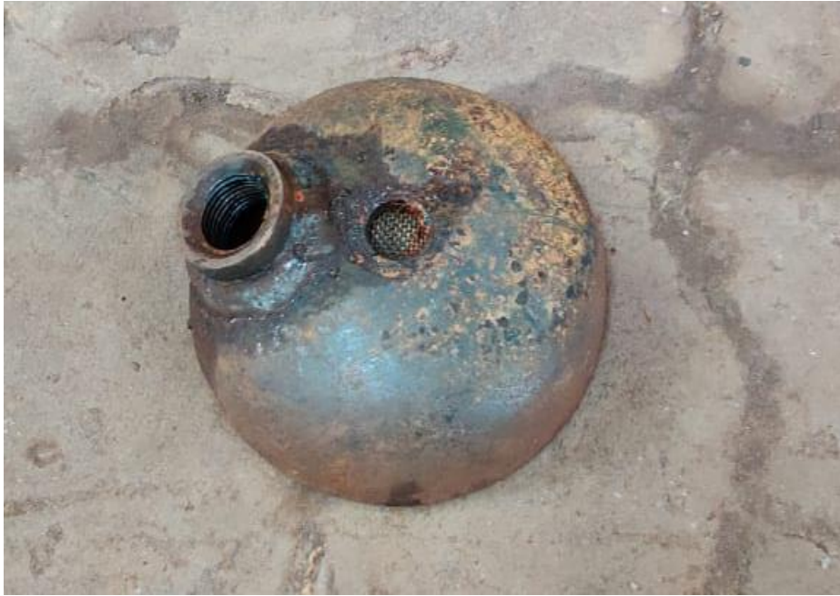
FIGURE 3. 14 External image showing crown of the tower with wire mesh seal to prevent desiccant carryover in the process line
