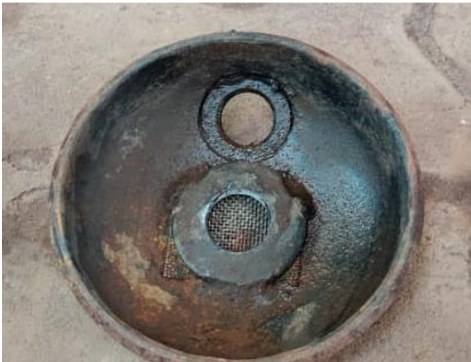
FIGURE 3. 15 Internal image showing crown of the tower with wire mesh seal to prevent desiccant carryover in the process line
