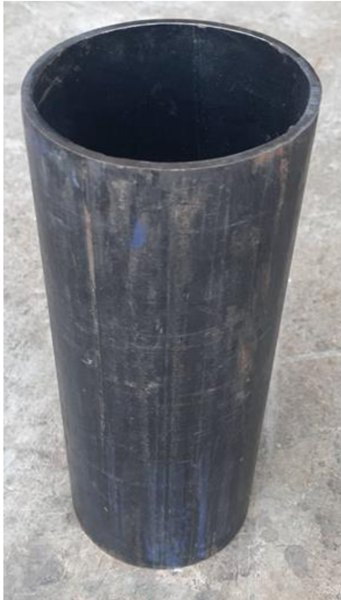
FIGURE 3. 13 Image of 4" diameter, 18 " height, 4mm thickness, SA1239 pipe used for tower fabrication.
