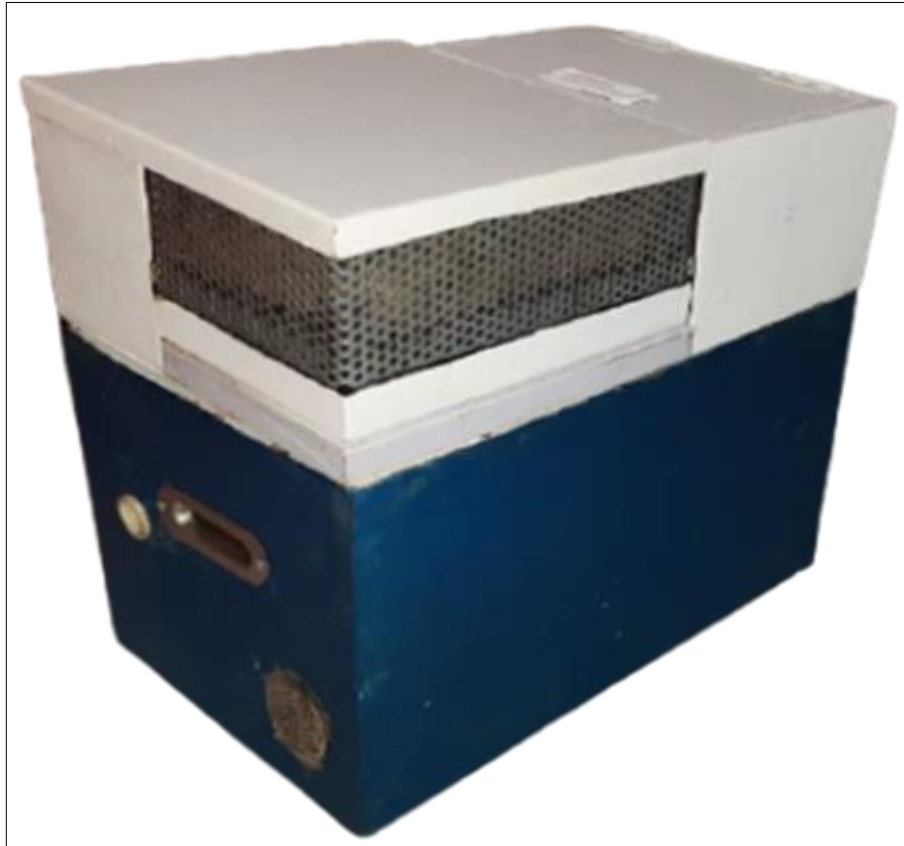
Figure 6.12 Complete prototype of evaporative cooling based BTMS
