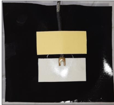
Figure 5.7 Backside of temperature sensor pasted on Vinyl adhesive tape
