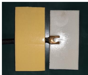
Figure 5.6 Temperature sensor pasted on foam tape
