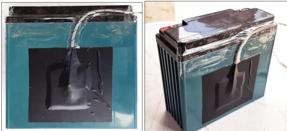
Figure 5.8 Temperature sensor pasted on the battery surface
