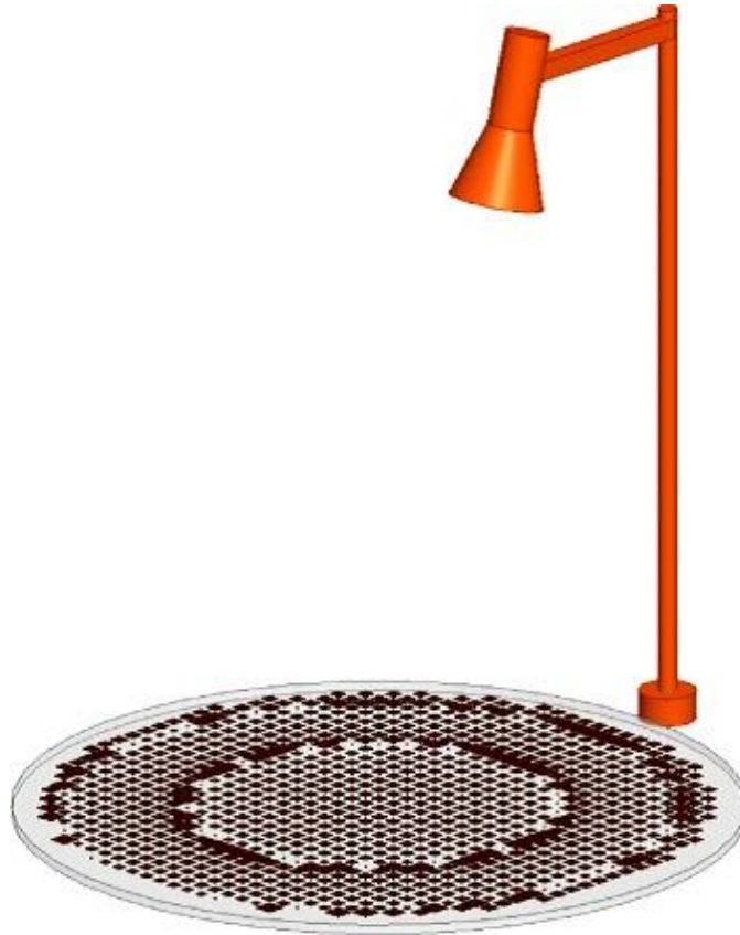
Figure 1: Geometry of offset fed reflectarray antenna
