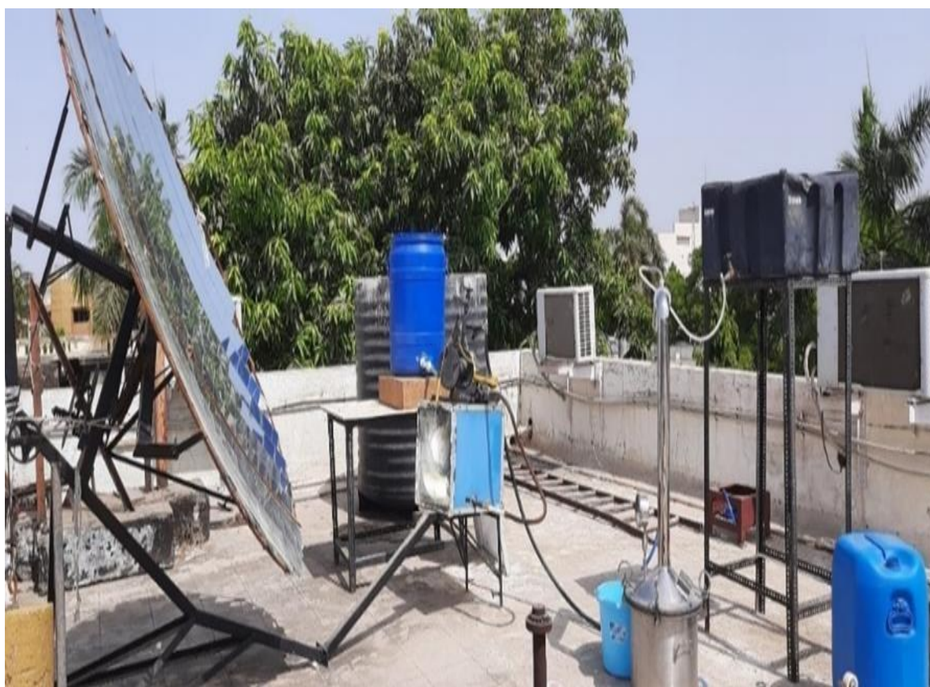
Figure 3. (a) Solar steam distillation system
