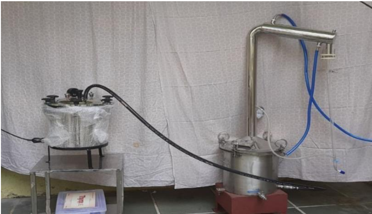
Figure 2. (a) Conventional electric-powered steam distillation system
