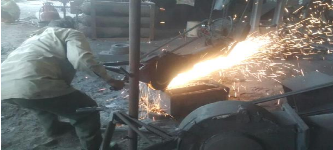
Figure 4.13. Grinding operation carried out in GTC to remove burrs and protrusions in the castings.
