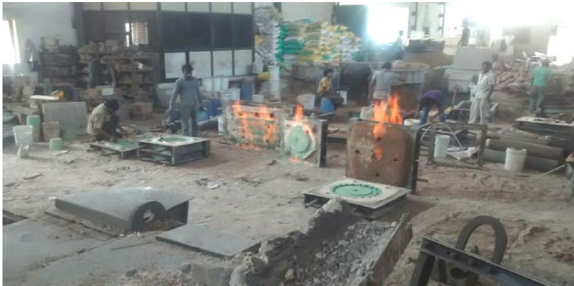
Figure 4.11. CO 2 moulding process in GTC
