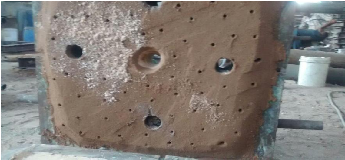
Figure 4.10. Vent holes made in a mould in GTC
