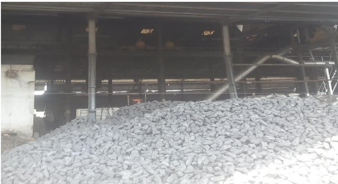
Figure: 5.28 Broken pieces of ingot mould/ scrap for charging material in Cupola furnace
