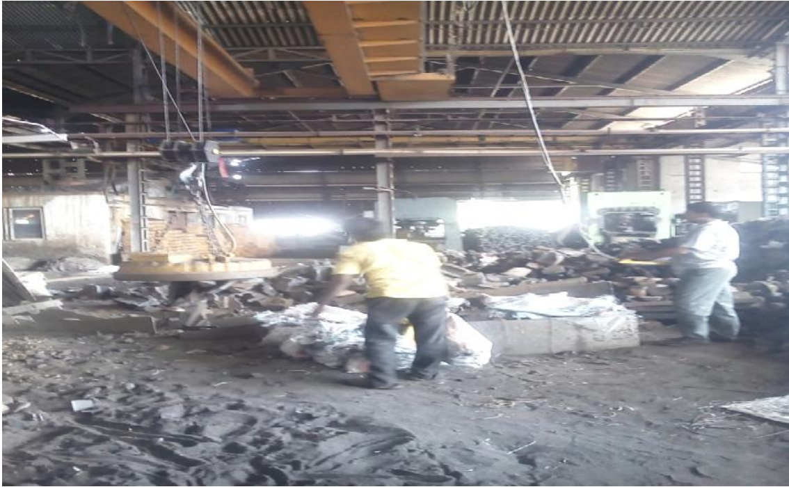
Figure: 5.27 Magnetic Separate overhead Crane
