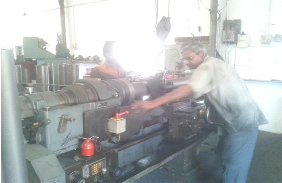
Figure 6.14. Rough turning operation carried in MF to remove burrs and protrusions in the castings
