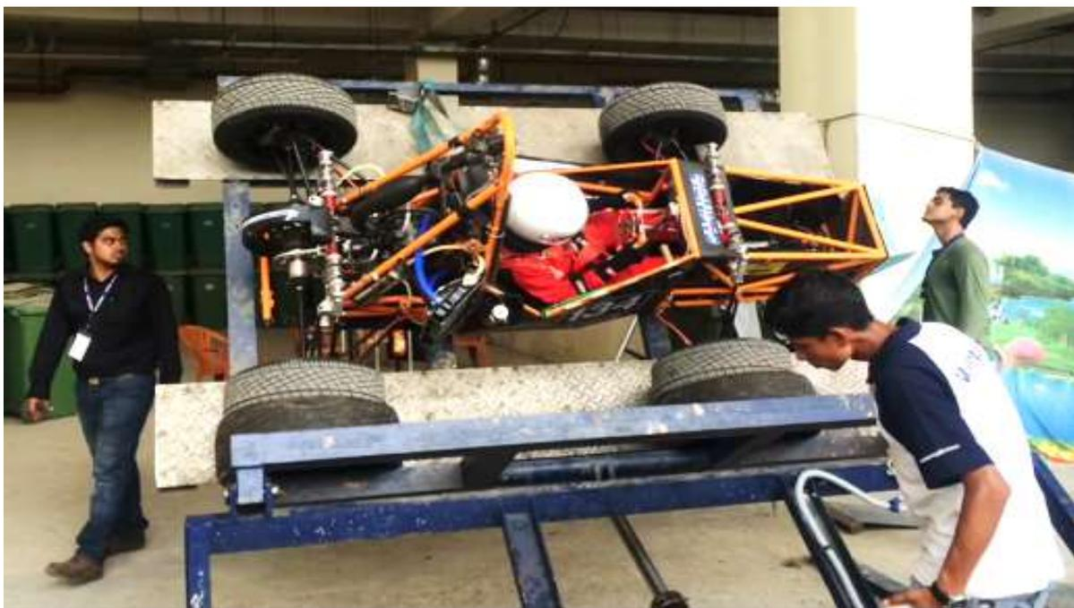
**A Car on Tilt Test Table**
