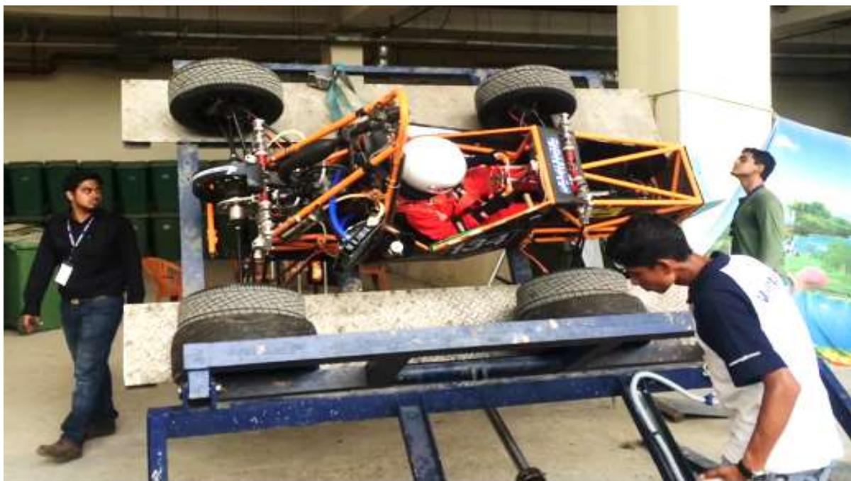
**A Car on Tilt Test Table**
