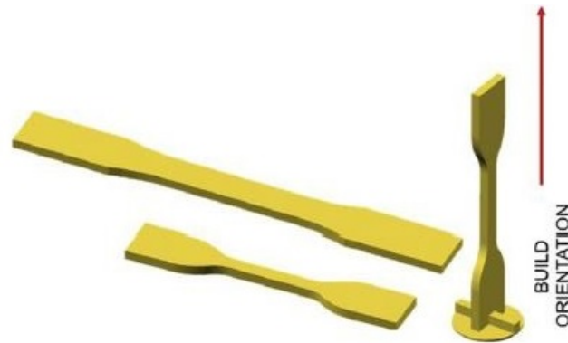
Figure 2.11: Tensile Specimens of ASTM D638-14 Type I vs. Type IV.
