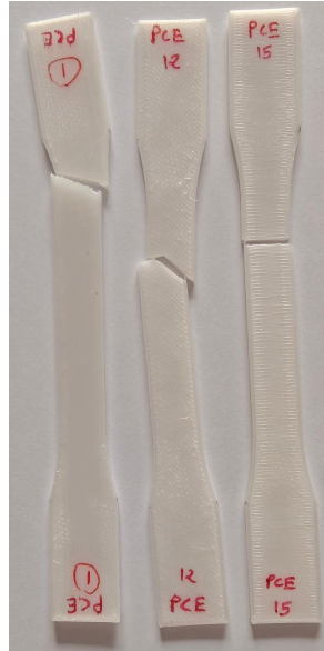
Figure 5.3: Tensile tested PC specimens with \theta = 0^\circ, 45^\circ, 90^\circ
