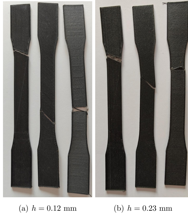
Figure 4.4: Tensile tested ASTM D638-14 specimens with \theta = 0^\circ, 45^\circ, 90^\circ (a) h = 0.12 mm (b) h = 0.23 mm
