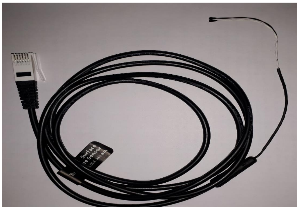
FIGURE 4.4 A thermal sensor for the recording of breathing pattern.
