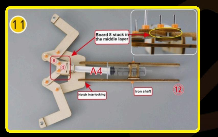
11. Clamp the (12) wooden pieces on to the A4 syringe through inserting a 5cm iron shaft through them and the syringe and secure the<mark>m w</mark>ith shaft sleeves on both sides.
