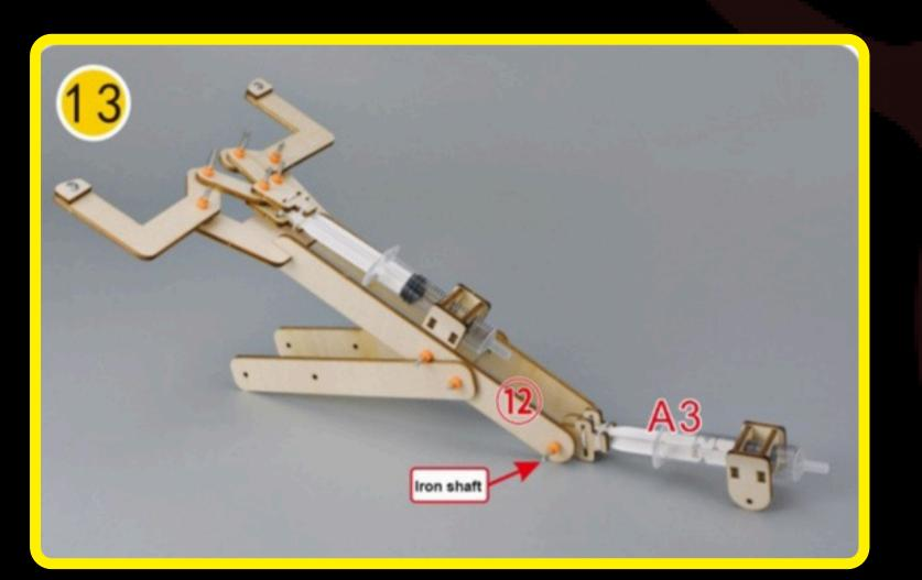
13. Connect the A3 syringe to the remaining end of (12)s using a 5 cm iron shaft and seal both sides with shaft sleeves.
