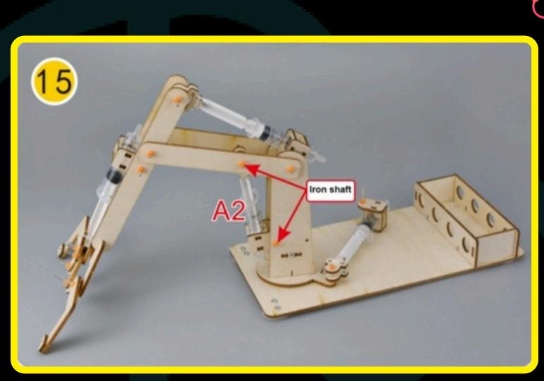
15. Install A2 syringe with the plunger inserted between (13)s and the syringe ring between (06)s.
