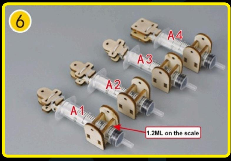
6. Use the four rings you prepared in step 4 and insert them onto the four syringes you prepared in step 5.
