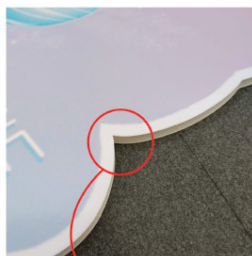
Overcut Effects May encounter many sharp edges that leads to overcut.
