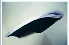
1. The thicker the booklet, the more the inner pages will creep out (extend out of cover size) when folded. Hence, keep vital elements of the layout for the inner pages away from the edges as much as possible to avoid them being trimmed off.
