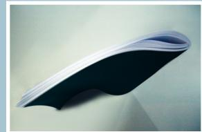
1. The thicker the booklet, the more the inner pages will creep out (extend out of cover size) when folded. Hence, keep vital elements of the layout for the inner pages away from the edges as much as possible to avoid them being trimmed off.
