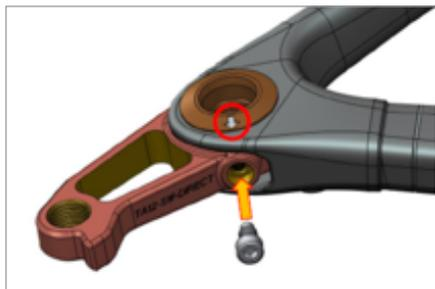
Make sure the location arrow is pointing to the lower bolt hole; insert the bolt (Max torque 1.5 N/M)
