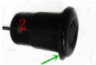
Install the first shim
