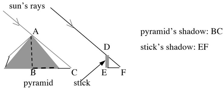
Thales needn't have waited till the shadow of the stick was of the same length as its height: he could have measured the shadow of the stick and the shadow of the pyramid at any time, and *calculated* the height of the pyramid from the height of the stick and the lengths of shadows of the pyramid and stick, using the formula:
