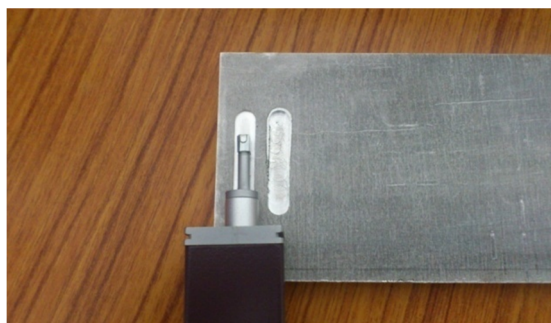
Fig 5.9 Roughness Measurement of optimization slots
