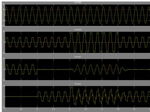
Fig. 7. Load voltage, load, grid, and DG currents before and after connection of DG and before and after connection and disconnection of additional load into the grid.
