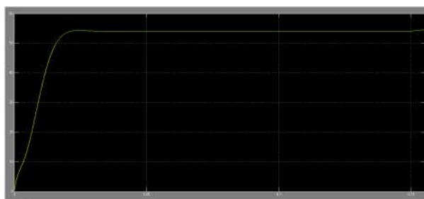
Fig. 7 voltage without boost converter
