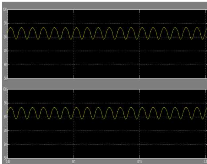
Fig 10 Experimental results for the dc-dc converter of the developed photovoltaic power generation system. (a) Voltage ripple of dc capacitor C2 (b) Voltage ripple of dc capacitor C3
