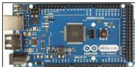
Fig.6. Arduino Mega 2560
